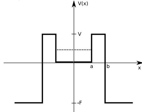
$$\begin{aligned} |x| < a : & \quad \psi(x) = \cos(qx) \\ a < |x| < a + b : & \quad \psi(x) = A \exp[-\kappa(|x| - a)] + B \exp[\kappa(|x| - a)] \\ |x| > a + b : & \quad \psi(x) = C \exp[ik(|x| - a - b)] \end{aligned} \quad (1)$$
