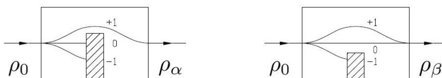
Figure 1: Stern-Gerlach devices ( \alpha ) and ( \beta ).
