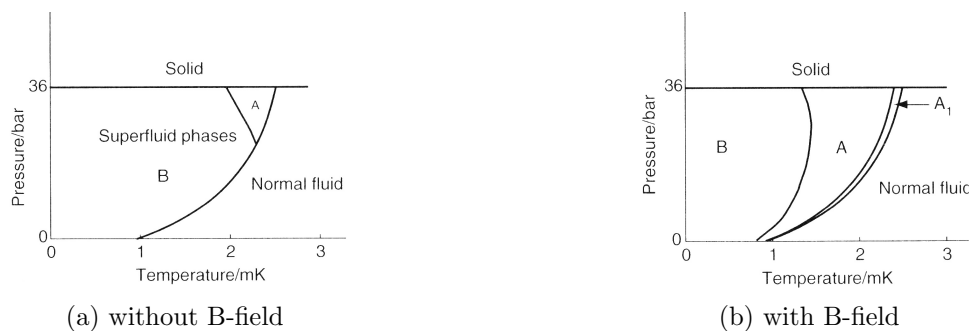
Figure 7.1: Phase diagram of ^3\text{He} (a) without and (b) with external B-field. From: Tony Guénault, Basic Superfluids.
