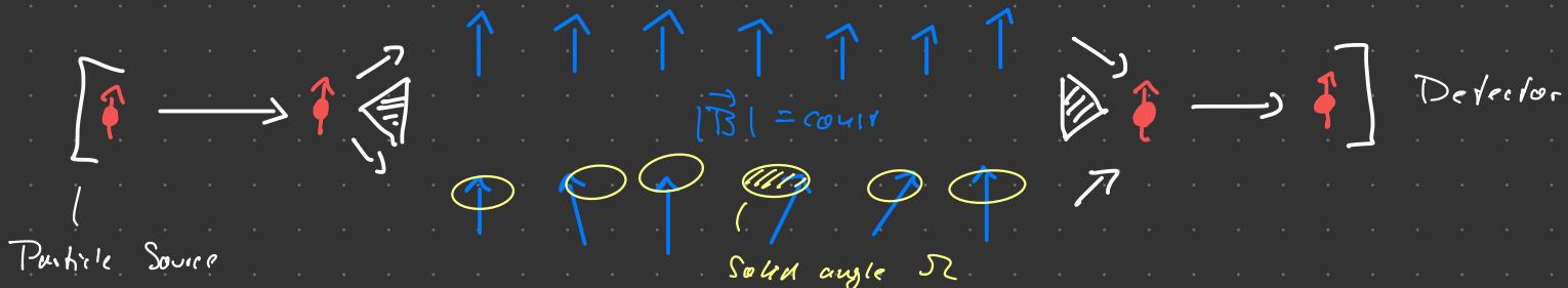
$$T\text{-Sel } 1 \Rightarrow e^{i\chi(p)} = e^{i\Omega/2} \quad (0 \leq \Omega \leq 4\pi) \rightarrow \text{Interference} \quad I = |1 + e^{i\chi(p)}|^2$$
